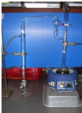
Figure 1 Protein extraction apparatus for vapor extraction of medicinal herbs.
